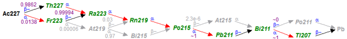
Figure 3. Details of the actinide decay chains modeled in the Clive DU PA Model, showing which species are omitted, in gray.
